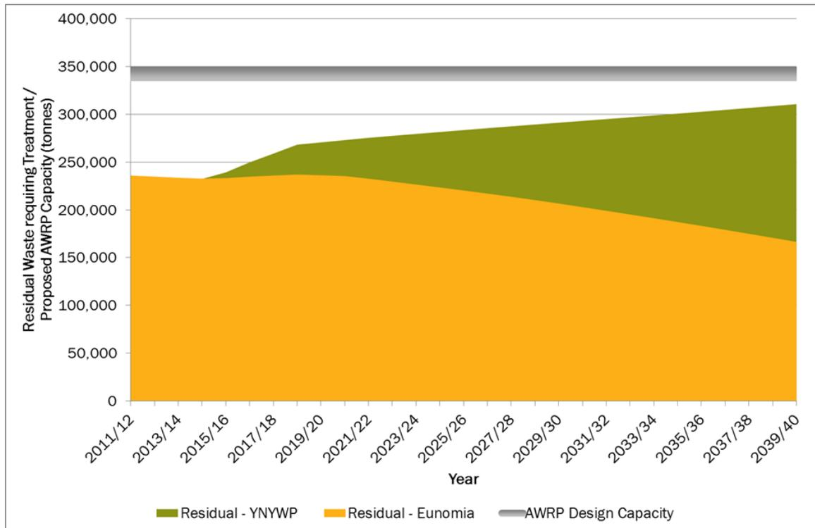
Note: The AWRP design capacity is presented as a range because the AmeyCespa Planning Statement suggests that although the incinerator will have a design capacity of 320 ktpa, it is more likely to operate at 305 ktpa
