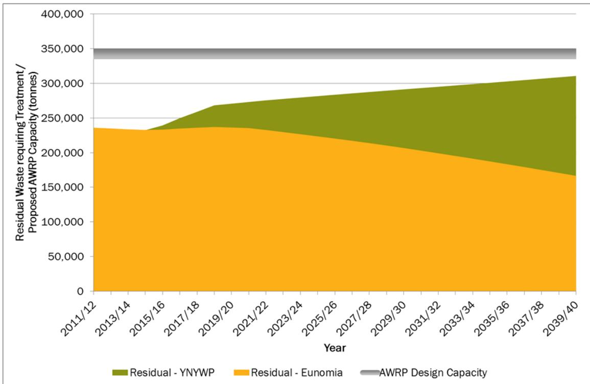
Note: The AWRP design capacity is presented as a range as the AmeyCespa Planning Statement suggests that although the incinerator will have a design capacity of 320 ktpa, it is more likely to operate at 305 ktpa
